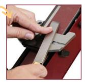
When the first side has been sharpened turn the skew over and place it against the other side of the jig and continue as before, until the tool is razor sharp.
